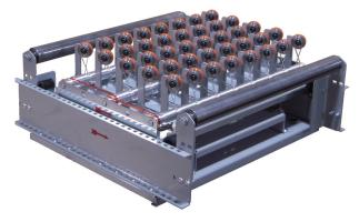
Reaching conveyor speeds of 350 fpm and a sort rate of 100+ cpm, Automotion's MB30 multi-belt sorter is both fast and accurate. In lieu of one wide belt, the MB30 utilizes multiple smaller width belts to carry product.
