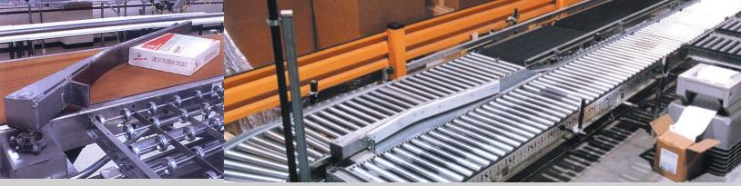
Mechanical Characteristics Nominal Conveyor Widths 24", 30" and 36"
