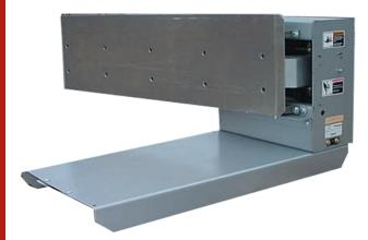
Automotion's High Speed Flat Face Arm Sorter can be used as an integral sortation component in almost any conveyor system. Our high speed induction conveyor strategically gaps and places the product onto the sortation belt conveyor. The High Speed Flat Face Arm Diverter is precision timed to swing out and make contact with the product to be sorted at a controlled rate of acceleration to provide a gentle sweeping divert action to a powered or non-powered takeaway conveyor.
