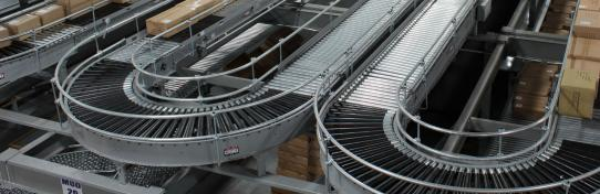
**Bed Section** 10" Deep x 1-3/8" Flange x 10 Gauge frame with 29-7/8" inside radius.
